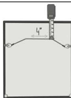
On the back of your frame, pull the wire up in 2 spots about 4" apart to simulate how it will hang on the hooks, then measure from the wire to the top of the frame.
