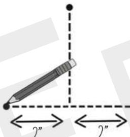
From the point you already marked on the wall, measure down whatever measurement you got in the last step. Mark 2" from each side of that spot.
