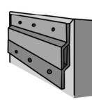
Slide the z bar on your frame over the Z bar on the wall and make sure they are lined up on the sides.
