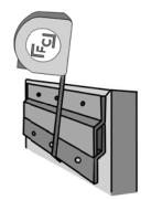
On the back of you frame slide your z bar under the Z bar already attached to the frame. Measure from the top edge of your frame down to the circular holes on your unattached z bar.
