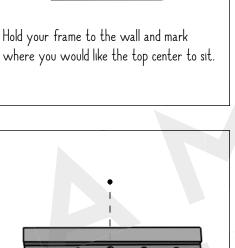
Hold your Z bar on the wall so that it is center with the mark and the holes are lined up with the mark.
